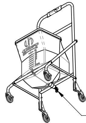
MODEL 9007 PORTABLE EYEWASH CART WITH TANK TANK DRAIN (1" BARB OR NPT)
