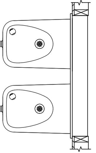
3/8" O.D. SUPPLY TUBING AND 3/8" O.D. PUSH-IN TEE SUPPLIED. (CONNECT TO FOUNTAIN SUPPLY LINE)
