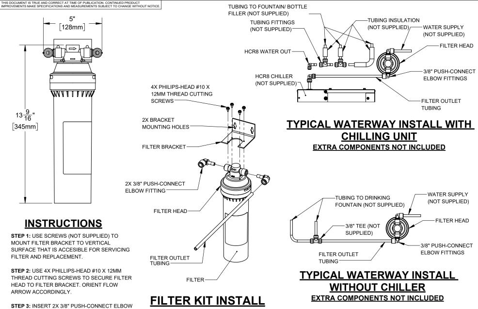
**STEP 4: INSERT FILTER INTO FILTER HEAD** ACCORDING TO NOTCHES ON INSIDE OF HEAD AND TOP OF FILTER AND MAKE 1/4 TURN UNTIL FILTER IS SECURE.
