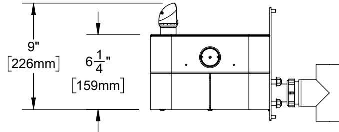
NOTE: STANDARD CONFIGURATION FOR MODEL 3670 ON A PEDESTAL IS SHOWN. IT IS RECOMMENDED THAT THE ASSEMBLY IS PLACED AT THE LOWEST OPENING ON THE PEDESTAL. THE MOUNTING PLATE CAN BE ROTATED SO THE DOG BOWL CAN BE IN A "HIGH" OR "LOW" POSITION. IT IS RECOMMENDED TO USE THE "LOW" POSITION AS SHOWN.
