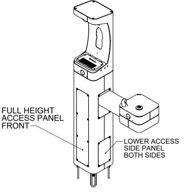
HAWS MODEL 3611/3611F IS FULLY COMPLIANT WITH THE FEDERAL 2010 AMERICANS WITH DISABILITIES ACT (ADA) ACCESSIBILITY REQUIREMENTS WHEN INSTALLED AS SHOWN HERE AND WHEN INSTALLED WITH PROPER CLEARANCES AND ACCESS. IT IS THE RESPONSIBILITY OF THE INSTALLER TO ADHERE TO LOCAL, STATE, AND FEDERAL CODES WHEN INSTALLING THIS UNIT. DISTANCE TO SURROUNDING OBJECTS, APPROACH SURFACES, ETC. SHOULD BE CONSIDERED. REFER TO SHEET 8 FOR MORE INFORMATION.
