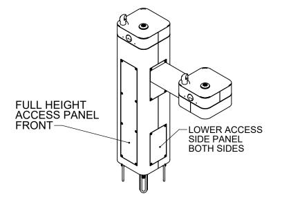
HAWS MODEL 3602/3602F IS FULLY COMPLIANT WITH THE FEDERAL 2010 AMERICANS WITH DISABILITIES ACT (ADA) ACCESSIBILITY REQUIREMENTS WHEN INSTALLED AS SHOWN HERE AND WHEN INSTALLED WITH PROPER CLEARANCES AND ACCESS. IT IS THE RESPONSIBILITY OF THE INSTALLER TO ADHERE TO LOCAL, STATE, AND FEDERAL CODES WHEN INSTALLING THIS UNIT. DISTANCE TO SURROUNDING OBJECTS, APPROACH SURFACES, ETC. SHOULD BE CONSIDERED. REFER TO SHEET 8 FOR MORE INFORMATION.
