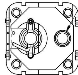
DRAIN OFFSET 2" TO ACCOMMODATE LARGER FILTER MAY BE REQUIRED. CHECK FOR FILTER CLEARANCES BASED ON THE OPTIONAL FILTER YOU PROVIDE, PRIOR TO SETTING DRAIN & ANCHORS.
