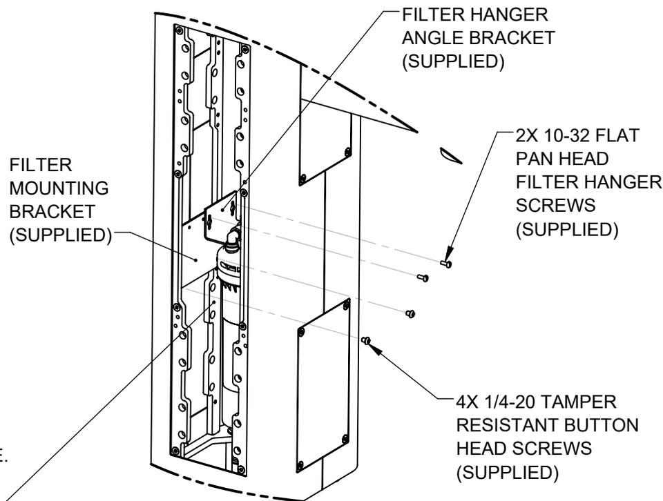
NOTE: FILTER BRACKET MOUNTS TO INSIDE OF THESE RAILS ON THE LEFT SIDE. USE THREADED HOLES SHOWN.
