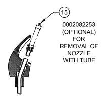
BUBBLER HEAD 5705 (TUBING CONNECTS TO INSERT ASSY)
