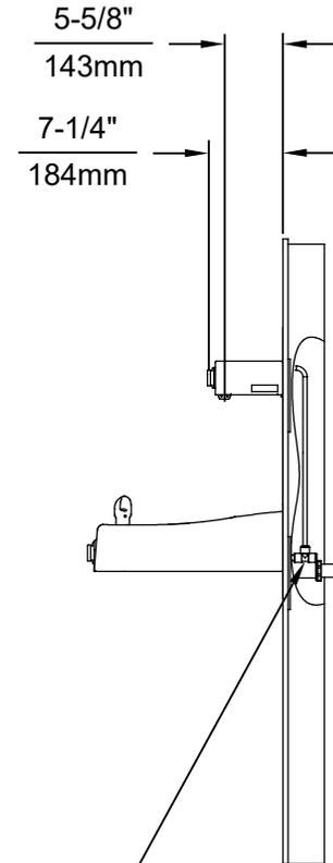
3/8" O.D. SUPPLY TUBING AND 3/8" O.D. PUSH-IN TEE SUPPLIED. (CONNECT TO FOUNTAIN SUPPLY LINE)
