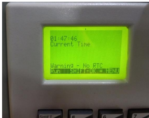
Figure 5. No RTC - Real Time Clock Display
