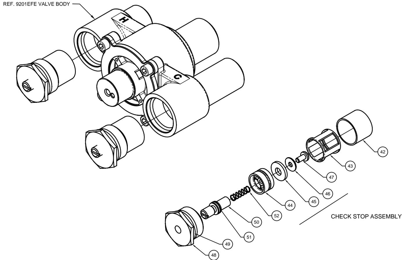
NOTE: HOT AND COLD CHECK STOPS ARE IDENTICAL. KIT INCLUDES BOTH.
