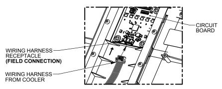
WIRING HARNESS CONNECTION (REAR OF BOTTLE FILLER)
