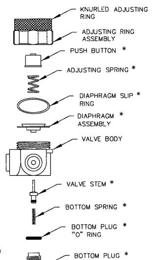
\* Indicated parts contained in VRK5872 repair kit.
