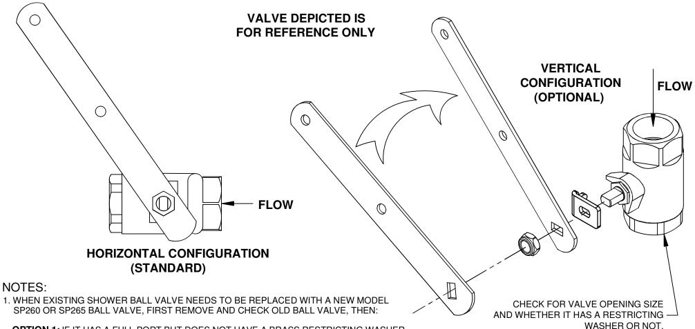
**OPTION 1:** IF IT HAS A FULL PORT BUT DOES NOT HAVE A BRASS RESTRICTING WASHER INSTALLED IN FRONT OF THE VALVE BALL, THEN JUST REPLACE IT.
