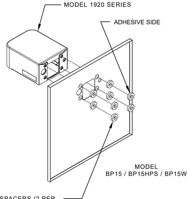
8 SPACERS (2 PER MOUNTING BOLT IF THE MOUNTING PLATE IS INSTALLED BEHIND THE FINISHED WALL. USE 1 SPACER PER BOLT FOR RETROFITS WHERE THE MOUNTING PLATE IS INSTALLED IN FRONT OF THE FINISHED WALL)
