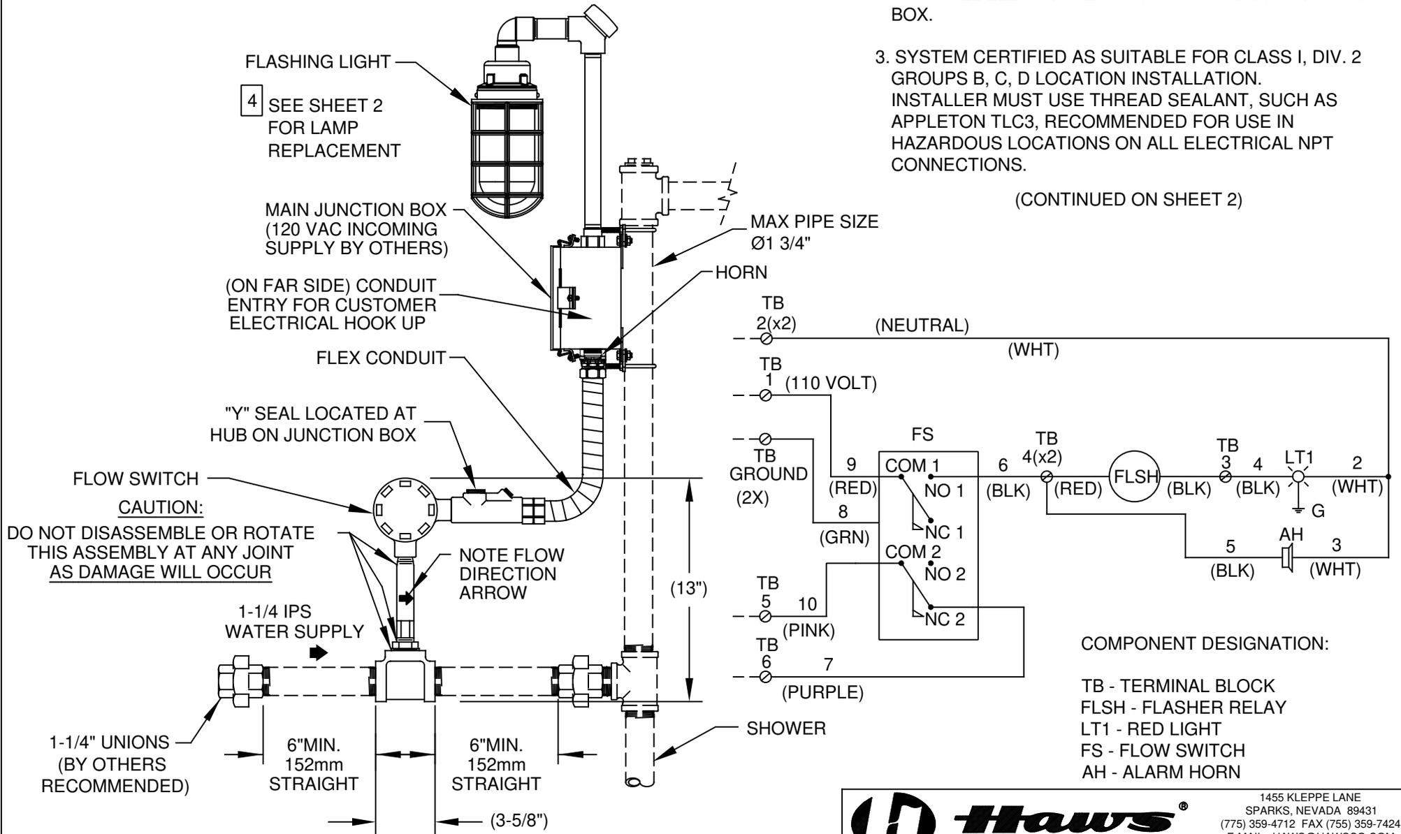
**SWITCH MUST BE MOUNTED IN HORIZONTAL POSITION**
