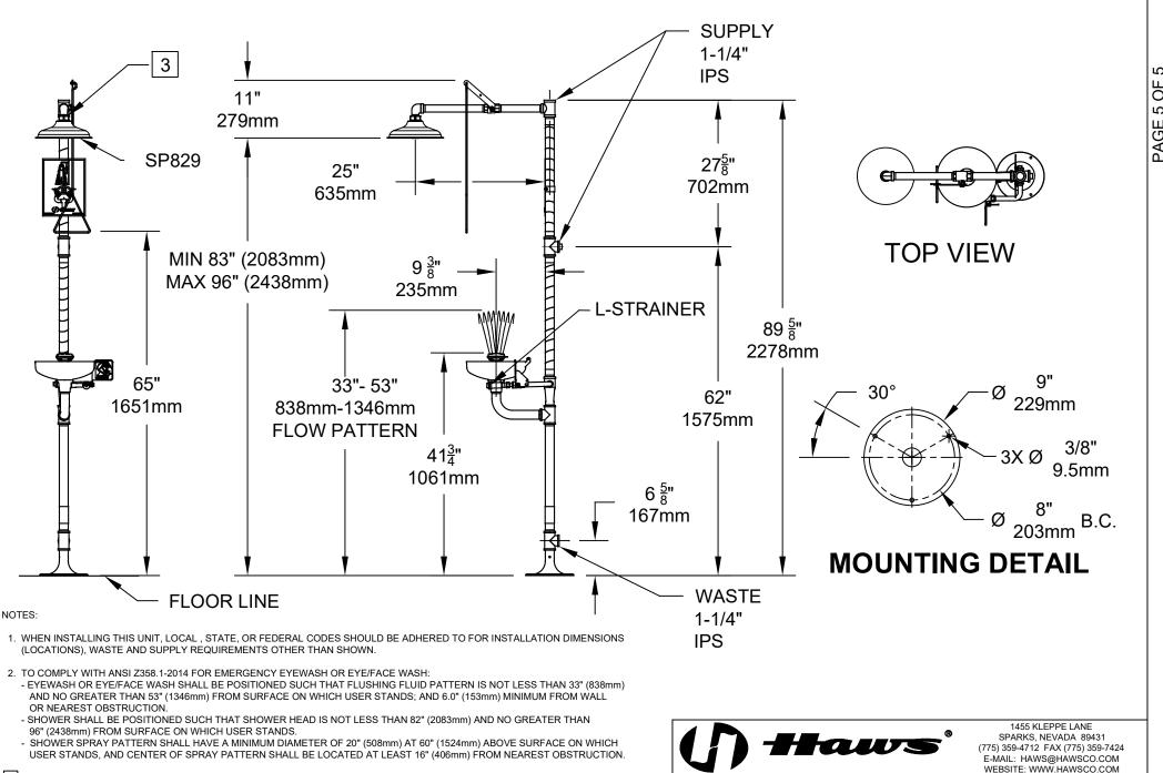
3 DO NOT USE REGULAR PIPE SEALANT. IF NECESSARY USE DOW CORNING 832 SEALANT PLACING FIVE SMALL BEADS ON THE MALE THREADS, JUST ABOVE THE FIRST THREAD.
