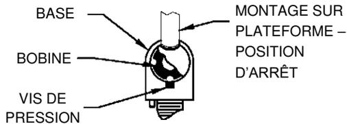
L'UNITÉ EST EXPÉDIÉE AVEC UNE CONFIGURATION DE MONTAGE SUR PLATEFORME. POUR CONVERTIR L'APPAREIL EN CONFIGURATION DE MONTAGE MURAL, PLACEZ LE LEVIER EN POSITION « DECK MOUNT OFF » (SANS MONTAGE SUR PLATEFORME) COMME CI-DESSUS.
