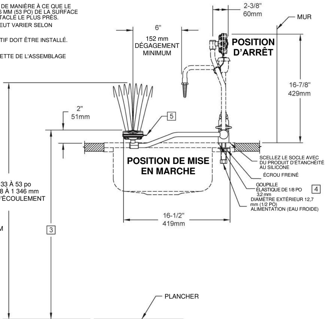
**CONFIGURATION DU MODÈLE 7610 MONTÉ SUR PLATEFORME**
