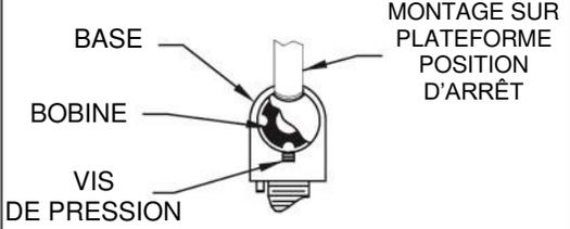
LE DISPOSITIF EST EXPÉDIÉ AVEC UNE CONFIGURATION DE MONTAGE SUR PLATEFORME. POUR LE CONVERTIR EN CONFIGURATION DE MONTAGE MURAL, PLACER LE LEVIER EN POSITION « DECK MOUNT OFF » (NON MONTÉ SUR PLATEFORME) COMME ILLUSTRÉ PLUS HAUT.
