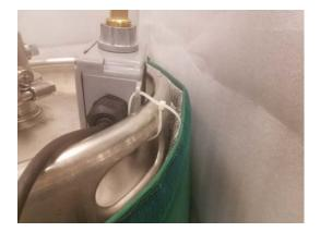
**STEP 8:** Attach grounding clamp to tank handle. Attach second ground clamp around metal hub on the junction box. Connect the two ground clamps with the supplied grounding wire.
