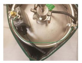
**STEP 9:** Attach conical top blanket with Velcro closures. Align the seam of the top blanket with the push flag. The electrical cord may exit across the Velcro seem at any location.
