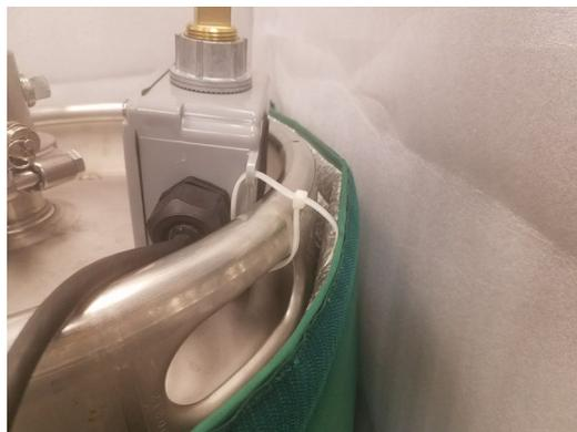
**STEP 7:** Attach grounding clamp to tank handle. Attach second ground clamp around metal hub on the junction box. Connect the two ground clamps with the supplied grounding wire.
