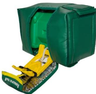
[Haws Model 7501T](#) is the only tempered portable eyewash on the market with a self-contained, 9-gallon, **gravity-fed, tempered eyewash**. The unit uses a heated, insulated blanket to provide ANSI-compliant tempered water in ambient operating temperatures from -30°F (-34°C) to 100°F (38°C) in non-extreme outdoor conditions. Ideal for remote locations without access to a continuous potable water source. Haz Loc and voltage options are available.
